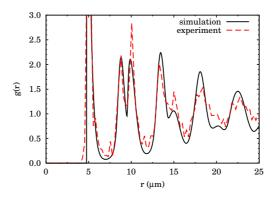
FIG. 2: Experimental radial distribution function *versus* simulated radial distribution function of the assembly of particles on the spherical droplet.
