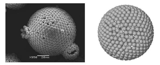
FIG. 1: Experimental colloidosome (on the left) versus simulated colloidosome (on the right)
