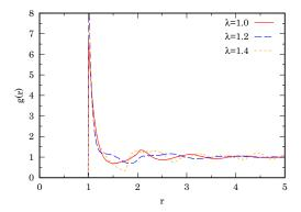
**Fig. 10** RDF for N = 100 HD of radius  $r_0 = 1$  with  $\epsilon = \sqrt{3}/2$  and  $\lambda = 1.0, 1.2, 1.4$ . The contact value for the  $\lambda = 1.2, 1.4$  cases is not shown. To be compared with Fig. 10 of Ref. [23]
