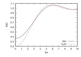
Figure 9. Structure factor for M = 4 and  $T^* = 0.1$ ,  $\eta = 0.1$  in the Bianchi *et al.* case using for the radial distribution function of the reference system,  $g_0$ , the zero density limit of the hard-sphere fluid. Also shown, for comparison, is the structure factor of the reference system,  $S_0(k) = 1 + 24\eta(k\cos(k) - \sin(k))/k^3$ .
