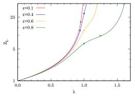
Fig. 1 Comparison between our MC (points) and the exact results (lines) of Ref. [22] for the longitudinal compressibility factor. The statistical error in the MC points is smaller than the point symbol. The MC simulations were up to  $10^9$  single particle moves long
