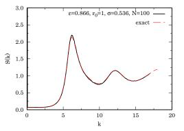
**Fig. 9** LSF for N = 100 HD of radius  $r_0 = 1$  with  $\epsilon = \sqrt{3}/2$  and  $\lambda = 1$ . We used  $2n_{\max} + 1$  wave numbers with  $n_{\max} = 270$ . The exact result in the thermodynamic limit, shared privately by A. Montero and not published before, fits our MC results very well
