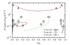
FIG. 3. (Color online) Comparison between the results of our numerical experiments (points from Table II) and of the laboratory experiments (lines from Table I in the Supplemental Material [21]) for the pressure-composition of three isotherms of the hydrogen-helium mixture phase diagram. A logarithmic scale is conveniently used on the ordinates. The double circled points at T = 15.5 K denote the case in which we observed gravity inversion in the numerical experiment.
