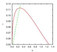
FIG. 6. (Color online) Phase diagram of our dipolarlike sticky hard spheres, calculated for defect energies  $\epsilon_1$ =0.186 and  $\epsilon_3$ =-0.0102. At the critical point the binodal curve (continuous line) and the connectivity transition (dashed curve) meet. The line denote the end-rich "gas" with the junction-rich "liquid."
