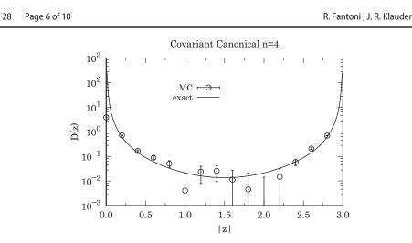
**Fig. 1** Two-point function D(z) of Eq. (3.2), for a free real scalar field subject to canonical quantization with a self-interaction potential density of the form  $V(\phi) = \frac{1}{2}m^2\phi^2$  in Eq. (1.1) with m = 1, N = 15, L = 3, a = L/N = 0.2. We compare with the analytic exact expression of Eq. (3.5) with an infrared cutoff of irc = 2. A logarithmic scale is used on the *y*-axis
