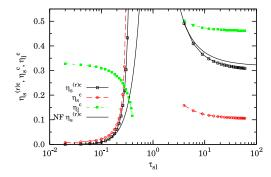
FIG. 10. Critical point for the fluid-fluid coexistence in the SAO model for  $q = q_0$  as a function of  $\tau_{sl}$ . The lines with symbols are obtained from perturbation theory, while the solid line corresponds to the NF criterion [see Fig. 9(d)]. A logarithmic scale is used on the abscissa. Equation (4.21) is used for the conversion between the reservoir and the solvent densities.
