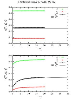
**Fig. 3.** (Color online) Critical point for the fluid-fluid coexistence in SSAO for q = 0.1 and  $\lambda_{sl} = 0.001$  (top panel) and  $\lambda_{sl} = (q_0 - q)/(1 + q)$  (bottom panel) as a function of  $T_c^*$ . The lines with symbols are obtained from thermodynamic perturbation theory, whereas the solid line corresponds to the Noro and Frenkel criterion of Fig. 2. Eq. (3.15) is used for the conversion between the reservoir density and the solvent density.
