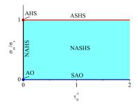
FIG. 3. Plane  $\sigma_{ss}/\sigma_s$  vs  $\tau_{sl}^{-1}$  sketching different models mentioned in the text. The general class of NASHS models includes, as limiting cases, ASHS ( $\sigma_{ss}/\sigma_s = 1$ ), SAO ( $\sigma_{ss}/\sigma_s = 0$ ), and NAHS ( $\tau_{sl}^{-1} = 0$ ). The intersection of the NAHS line with the ASHS and SAO lines defines the AHS and AO models, respectively. In this paper, we will be concerned with the ASHS and SAO models.
