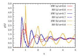
Fig. 12 LDF for N=100 SW/SS cases a with  $\sigma=6/10,7/10$  and b with  $\sigma=6/10$
