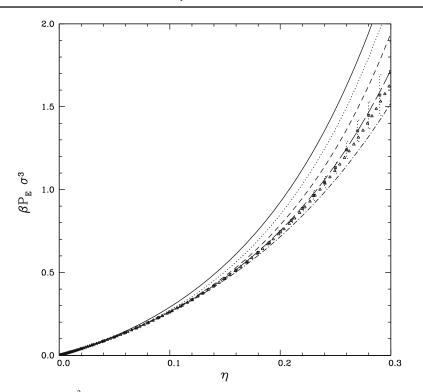
**Fig. 5** We show  $\beta P \sigma^3$  as a function of the packing fraction at  $\tau = 1$  for various approximations: MSA (*continuous line*), C0 (*dotted line*) [10], C1 (*short dashed line*) [10], PY (*long dashed line*) [9], AWC 1st order (*dotted dashed line*), AWC 2nd order (*empty squares*), and Monte Carlo results of Miller and Frenkel (*empty triangles*) [11].
