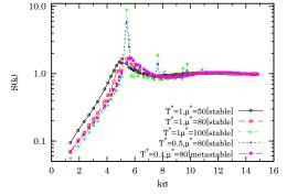
Fig. 2. Static structure factor  $F_k(0) = S(k)$  at  $\lambda^* = 1$  and  $T^* = 1, \mu^* = 50$  (stable), 80 (stable), 100 (stable) and  $T^* = 1/2, \mu^* = 80$  (stable), 80 (metastable). On the ordinates axis we use a logarithmic scale.
