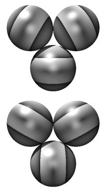
FIG. 6. Configurations of three mutually bonded spheres, each possessing two patches (dark shading). In the upper panel only one patch on each sphere is involved in the bonds; in the lower panel both patches on each sphere are involved. The latter case is only possible for  $\delta \ge \pi/3$ . Combinations of these arrangements are also possible.
