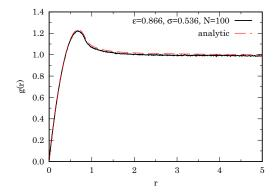
Fig. 7 RDF for the ideal gas with  $\lambda = 1$  and  $\epsilon = \sqrt{3}/2$ . Here, the g(r) is calculated from Eq. (2.6) using for  $n_{\rm id}(r)$  its asymptotic value  $2\lambda\Delta$  everywhere. The analytic result is the one in the thermodynamic limit of Eq. (3.1). The slight discrepancy is the expected finite size effect. Remember that  $\lim_{r\to\infty} g_{\rm id}(r) = 1 - 1/N$
