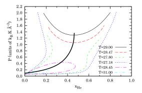
FIG. 1. (Color online) Schematic pressure-composition phase diagram for six isotherms of the hydrogen-helium mixture at low temperatures and low pressures as obtained in the experimental work by Streett *et al.* [4]. The thick continuous black line is the mixture critical line.
