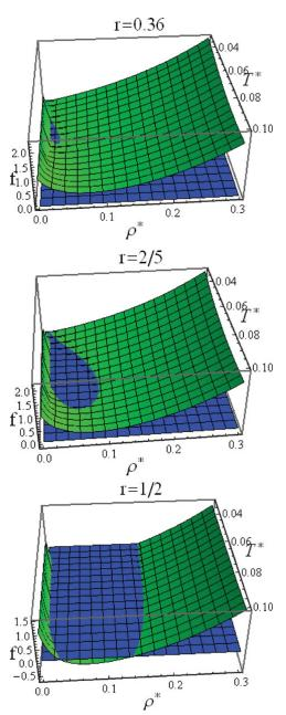
Figure 5. Tridimensional plots of  $f(T, \rho; r) = d\beta p/d\rho$  (green surface) for r = 0.36, 2/5, 1/2 from top to bottom. Also, shown is the plane f = 0 (blue surface). For r = 1/3, the two surfaces become tangent at small temperatures and small densities. For r > 1/2, the minimum in the pressure moves at larger densities at smaller temperatures.
