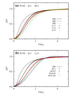
Fig. 2 The radial distribution function for Jellium in selected states of Table 1, from algorithm A, at fixed temperature in the upper panel (a) and at fixed density in the lower panel (b). Also shown is the Debye–Hückel (DH) result [39] for the high temperature and low density limit,  $g_{\rm DH}(r) = \exp\left[-\frac{\Gamma}{r}\exp\left(-\sqrt{3\Gamma}r\right)\right]$
