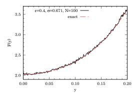
**Fig. 4** TDP for N = 100 HD with  $\epsilon = 0.4$  and  $\lambda = 0.671w$ . The exact result, shared privately by A. Montero and not published before, fits our MC results very well. In particular from Fig. 4 of Ref. [22], we see how the particles tend to escape from the center of the channel preferring to stay in contact with the walls as density approaches the packing density
