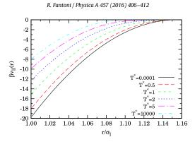
**Fig. 1.** (Color online) Effective potential for the SSAO mixture at various reduced temperatures and q = 0.1,  $\lambda_{sl} = (q_0 - q)/(1 + q)$ ,  $\eta_s^{(r)} = 1/2$ .
