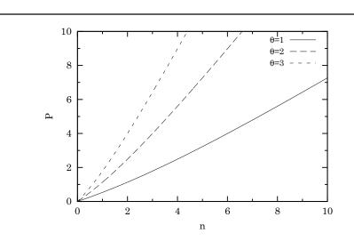
Fig. 1 The equation of state for the Lenard's model at various temperatures  $\theta$  for q = 1
