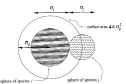
FIG. 1. Schematic diagram showing the area of the contact surface between a particle of species i and a particle of species j.
