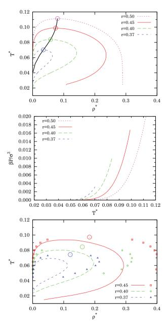
Figure 4. Top panel: evolution of the gas—liquid binodal as a function of r. The continuous thick black line is the locus of the critical points for  $r \in ]1/3$ , 1/2]. Middle panel: pressure—temperature diagram. Bottom panel: binodals of Russo *et al.* [7] Figure 4 as obtained from their analysis (lines) of the Wertheim theory and from their MC simulations (points); the big circles are their predicted critical points.
