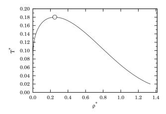
Figure 1. Gas-liquid binodal for the HS plus the van der Waals mean-field term. The circle is the critical point at  $\rho^*$ 0.249129,  $T_c^* \approx 0.180155$ , and  $z_c \approx 0.358956$  [34].
