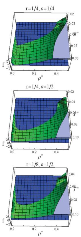
Figure 8. Tridimensional plots of  $f(T, \rho; r, s) = d\beta p/d\rho$  (green surface) for (r, s) = (1/4, 1/4), (1/4, 1/2), (1/8, 1/2). Also shown is the plane f = 0 (blue surface). As we can see, the spinodals of the two cases (r, s) = (1/4, 1/2), (1/8, 1/2) look essentially the same.
