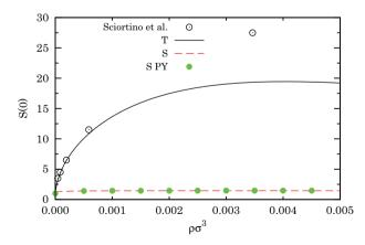
Figure 10. Structure factor at zero wave-number as a function of density for M=2 and  $T^*=0.055$  in the Sciortino *et al.* simulations of Ref. [4], from the thermodynamic route (T) of the isothermal compressibility of Equation (58), from the structure route (S) of Equation (55), and from the zero wave-number limit of Equation (54) taking as a reference system the Percus–Yevick analytic solution for hard-spheres (S PY).
